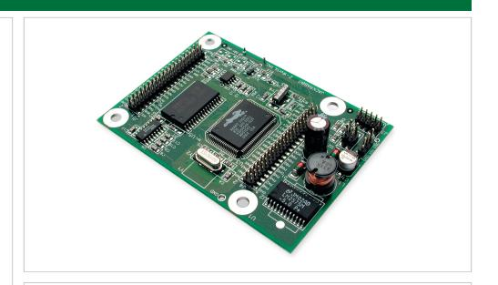
The BL1800 Jackrabbit is a small, easy-to-use, single-board computer that offers reliable hardware for embedded applications.
